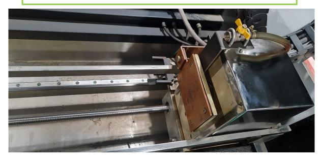
Optional Servo driven Magnetizing Coil for automatic multiple coil shots
