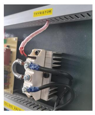
Thyristorized current control - stepless control with Feedback system - Ensures delivery of set currents within the range of +/\_ 10% with an alert to the operator
