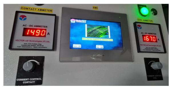
Digital Ammeters with memory retention - will retain the reading till the next
