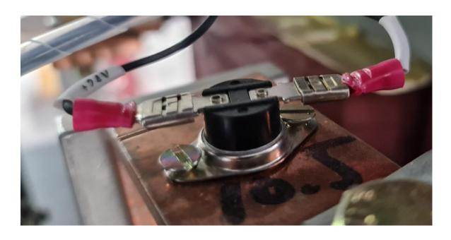
**Transformer Overload Protection & alarm**
