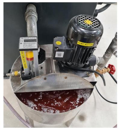
Bath Pump with controlled agitation system
