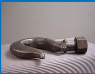
Crane Hook with Service Induced Crack
