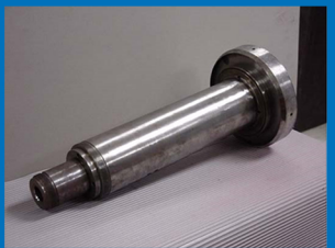
Drive Shaft with Heat Treatment Induced Cracks
