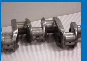
Crank Shaft with Service Induced Crack Near Lube Hole
