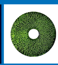
Rocker Arm Raw Material Crack
