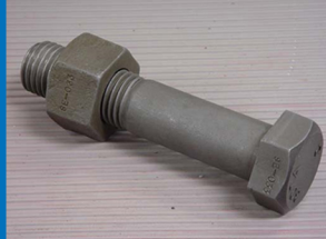
Large Bolt with Service Induced Crack
