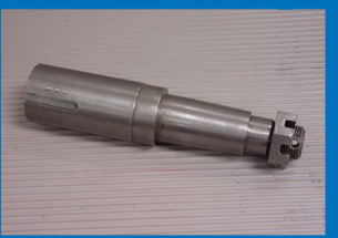
Threaded Shaft with Service Induced Crack
