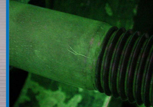
Large Bolt with Service Induced Crack
