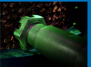
Threaded Shaft with Service Induced Crack
