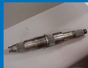
Splined Shaft with Service Induced Cracks
