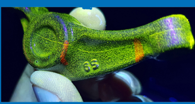
Rocker Arm Raw Material Crack
